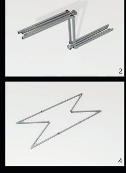
**HONOCLIP 32 1-7** Open the folded frame horizontally and the locking hinges quickly engage and lock automatically. Pull the frame apart and the vertical frame parts lock into place.
