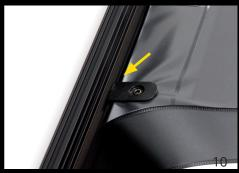
The surface is attached to the frame at the circumferential slot with its hooks.Middle struts or other support elements are mounted afterwards. See point 16 to 22.
