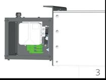
**3** In order to get access to the cam unit, remove the cover (green) of the rotary limit switch. (Phillips or slot screwdriver).
