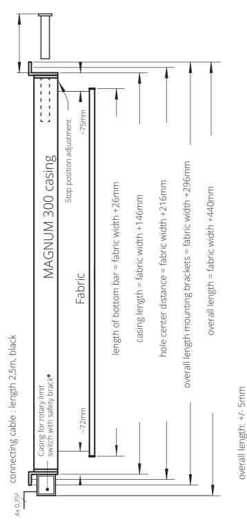
\* For servicing and adjusment of the rotary limit switch and safety brack the casing must be accessible at least from the front and the bottom.
