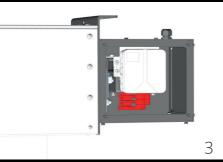
**3** In order to get access to the cam unit, remove the cover (red) of the rotary limit switch. (Phillips or slot screwdriver).
