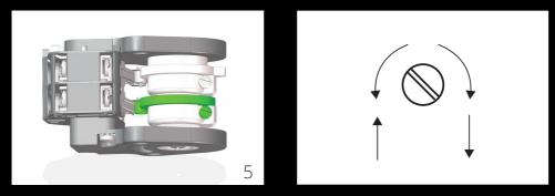
**5** The stop point for the lower emergency limit switch is set by means of the set screw at the lower switching cam (green).
