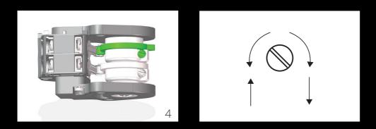
**4** The stop point for the upper emergency limit switch is set by means of the set screw at the top switching cam (red).
