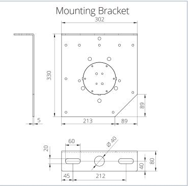
THE BRACKETS OF THE PROJECTION SCREEN MUST BE MOUNTED FORCE-FIT AND POSITIVE-FIT TO THE CEILING CONSTRUCTION! DO NOT PUT ADDITIONAL MECHANICAL LOAD ON THE CASING! THE MOUNTING MUST ENSURE THAT NO DISTORTION CAN ARISE!
