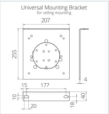
THE BRACKETS OF THE PROJECTION SCREEN MUST BE MOUNTED FORCE-FIT AND POSITIVE-FIT TO THE CEILING CONSTRUCTION! DO NOT PUT ADDITIONAL MECHANICAL LOAD ON THE CASING! THE MOUNTING MUST ENSURE THAT NO DISTORTION CAN ARISE!
