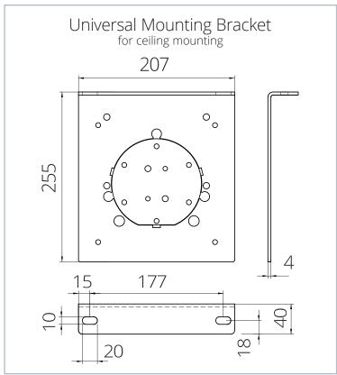
THE BRACKETS OF THE PROJECTION SCREEN MUST BE MOUNTED FORCE-FIT AND POSITIVE-FIT TO THE CEILING CONSTRUCTION! DO NOT PUT ADDITIONAL MECHANICAL LOAD ON THE CASING!
